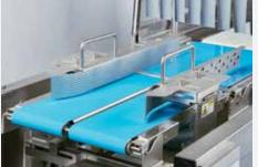
Products are automatically separated for optimum performance, and aligned with the self-positioning guides to enable accurate label placement.
